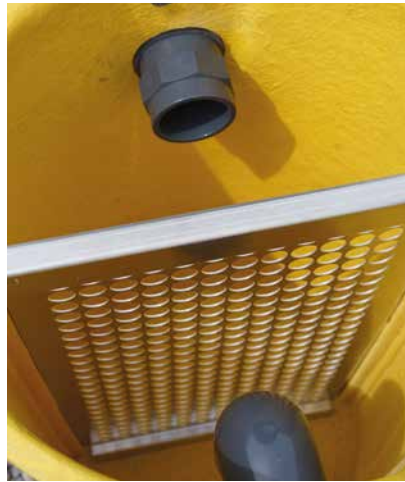
Filtration with the perforated stainless steel filter sieve
