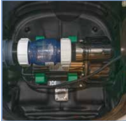
Check valve and sewage pump Torpedo
